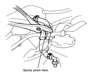
If there is no clicking sound, check the PCV valve grommet for cracks or damage. If the grommet is OK, replace the PCV valve and recheck.
