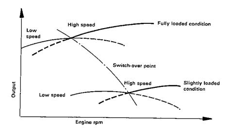
The above graph shows changes in the switch-over point in relation to engine rpm and load.
