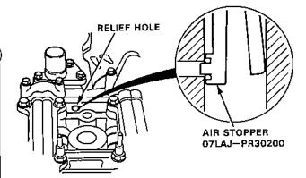
Remove the bolt and washer from the inspection hole and connect the special tool (Valve Inspection Set).
