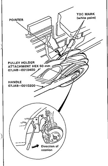
NOTE: If the pully bolt loosens while turning the crank, retorque it to 120 N·m(12.0 kg-m, 87 lb-ft).
