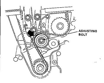
25. Remove the timing belt from the camshaft pulleys.
