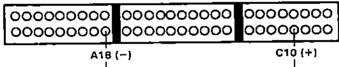
Measure voltage between C10 (+) terminal and A18 (-) terminal.
