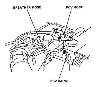
At idle, make sure there is a clicking sound from the PCV valve when the hose between PCV valve and intake manifold in lightly pinched with your fingers or pliers.
