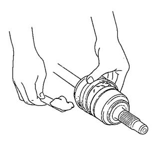
Adjust the length of the driveshafts to the figure below, then adjust the boots to halfway between full compression and extension.
