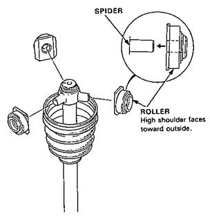
Pack the inboard joint with molybdenum disulfide grease.
