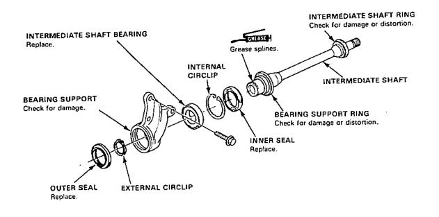
CAUTION: Be careful not to damage the rubber on the bearing support during installation.
