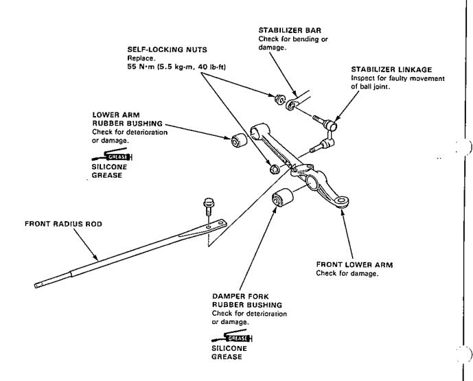
CAUTION: The vehicle should be on the ground before any bolts or nuts connected to rubber mounts or bushings are tightened.
