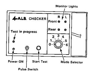
With the transmission in neutral, rotate each wheel briskly (one revolution per second) by hand and confirm that its respective monitor light on the checker blinks as the wheel rotares.
