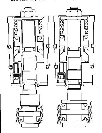
Adjust so that the brake fluid flows into the piston mounting hole in the modulator body.
