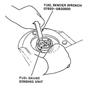
Measure the resistance between the A and B terminals at E (EMPTY), 1/2 (HALF FULL) and F (FULL) by moving the float.
