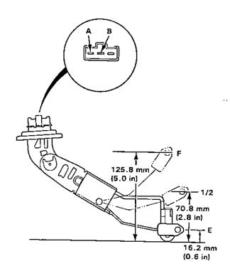
If unable to obtain the above readings, replace the fuel gauge sending unit.
